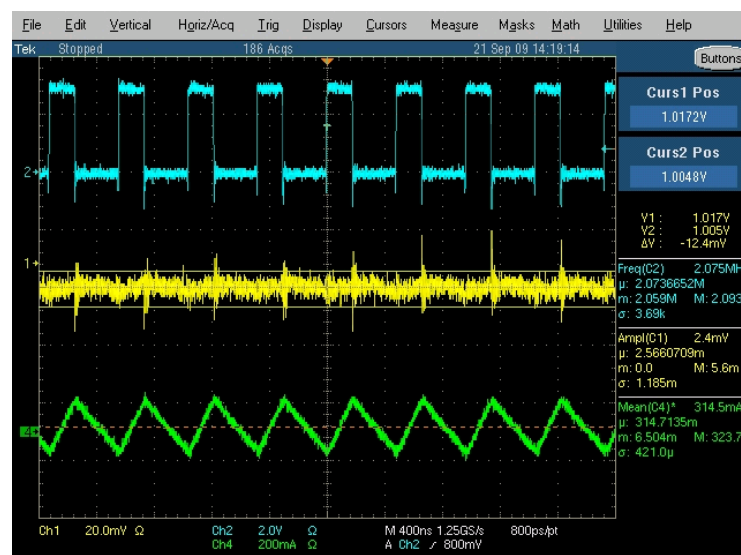
Figure 14. L=GLK2510P-2R2M, C=Ceramic 4.7 \mu F 0805 X5R TDK (Ripple 12.4mV)
