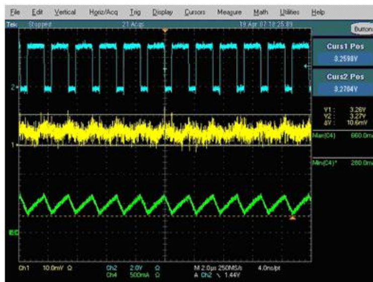
Figure 13. Ceramic 10 \mu F 0603 (X5R) (Good)
