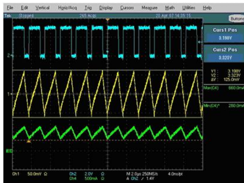
Figure 20. Electrolytic 100 \mu F (Ripple Too High)
