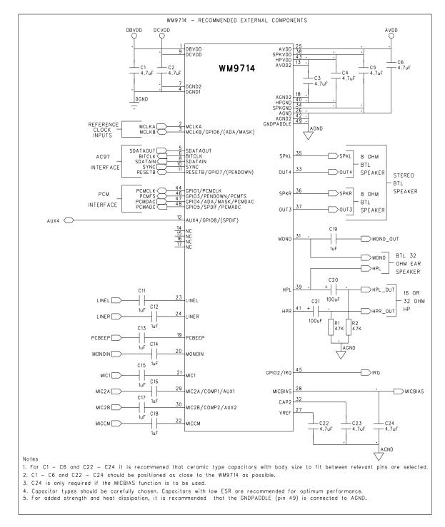
Figure 28 Recommended External Component Diagram
