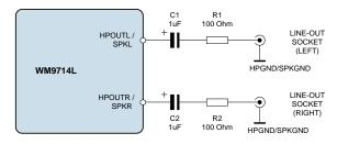
Figure 29 Recommended Circuit for Line Output
