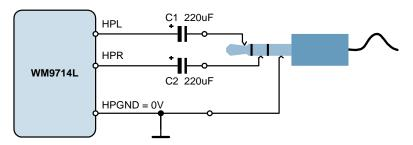
Figure 30 Simple Headphone Output Circuit Diagram
